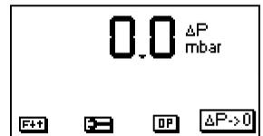
Different functions can be called up with the function key <F1>. The current seizure of the other function keys (<F2> - <F4>) is shown on the display. Press one time <F1> to display the functions „Hold“, „Min/Max“ and „Print“.
