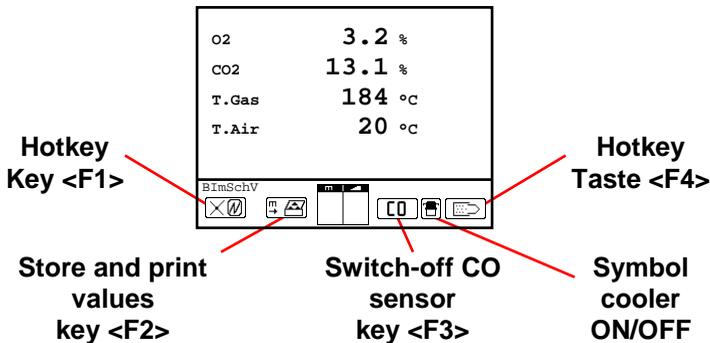
Pressing <F1> enables to switch, from the values display, to a menu point selected before or on „Standby“ (see chapter Adjustments). Possible menu points are: Soot...Oil trace, Data processing, View memory, Display values, Fuel type, Efficiency (K), Internal, Adjustments. Furthermore you can switch back from any random menu point to the values display with <F1>.
