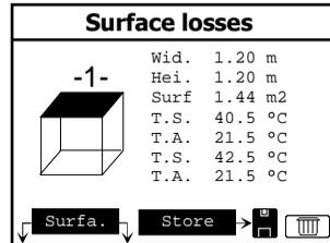
Once all surface temperatures have been determined, quit the menu with **<ESC>**. The surface losses get automatically calculated. The value conversion in negative points is available in the menu point „**Results**“.
