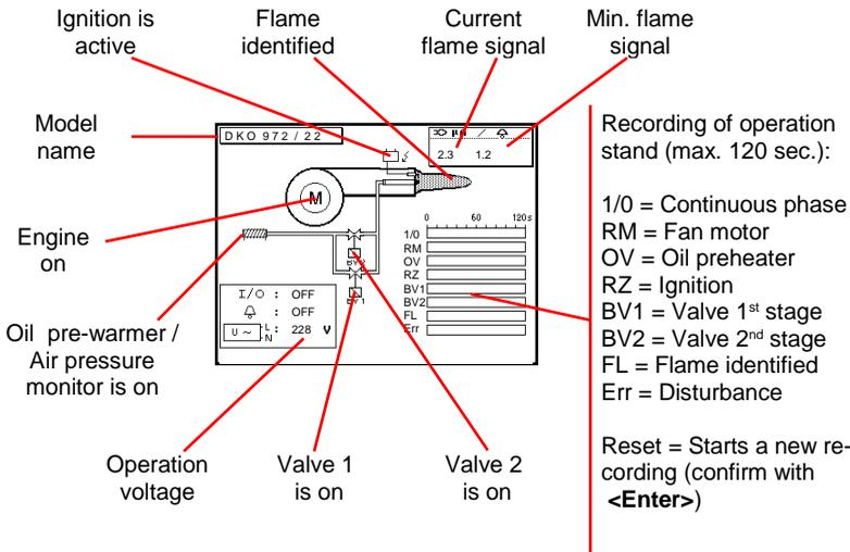
Use the cursor keys (Up/Down) to call up further data of the firing automate. On the 2<sup>nd</sup> display page the current error and the number of burner starts are displayed.
