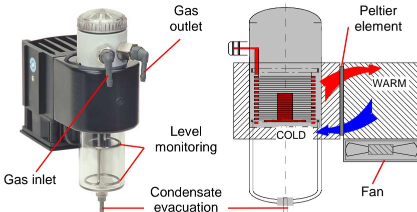
Exhaust gas with a temperature over the steam dew point (35 - 65 °C) is flown spiral via a long gas path thru a surface coated metal body with good thermal conductivity. The gas radiates its heat to this metal body. A Peltier element (semi-conductor cooling element) flown by a continuous current is thermal connected with this body and with a second metal body with cooling ribs and ventilation slots.
