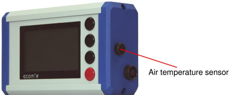
If there is no air temperature sensor connected at the ecom-EN2, then the air temperature sensor of the ecom-R supplies the measured values.
