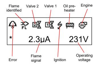
**2. Flame signal** (current flame signal - minimum signal)
