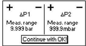
After switch-on, the specifications of the pressure sensor will be displayed: denomination, measurement range and connection seizure (+/-). Press <OK> to access to the measurement value menu.
