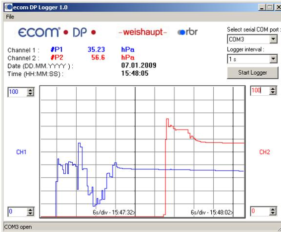
The measured value process of the **ecom-DP** can be logged with the help of the data logger program „ecom-DP Logger “. The program can be loaded free of charge from the download area of the ecom homepage [www.ecom.de](http://www.ecom.de). To transfer the data a USB cable (kind becomes. - No.: 55818) and a driver (free download from [www.ecom.de](http://www.ecom.de)) is needed. The measured value rows can be stored in the xls format (Excel).
