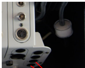
Connections for pitot tube
