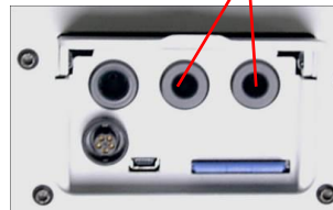
Connections for pitot tube
