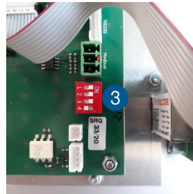
1 Knurled screw 2 Front plate 3 DIP switch
