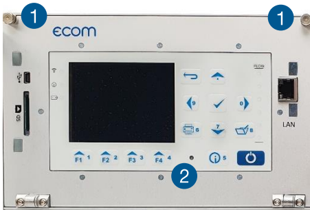
1 Knurled screw 2 Front plate 3 DIP switch
