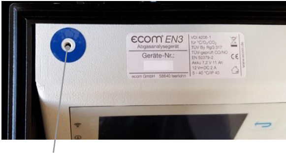
Fresh air opening
