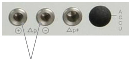
Connections for Pitot tube
